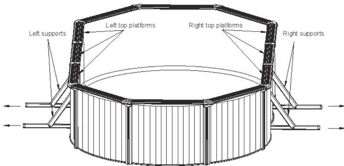
Make sure the top platforms are in a line by moving the supports.
